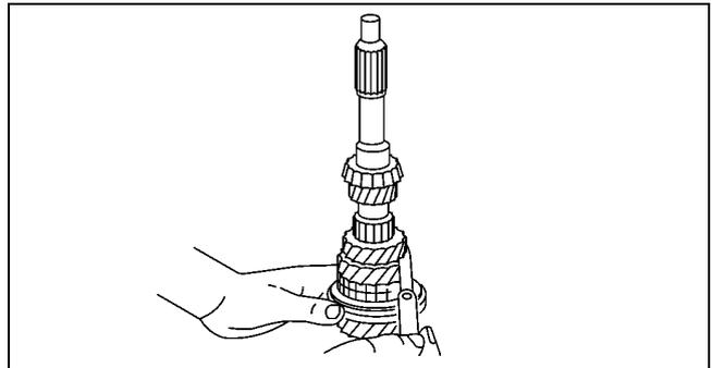
3. Measure the clearance between the 4th gear and bearing.
